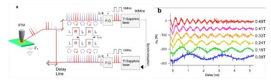
**Fig.1.** (a) The schematic of the OPP-STM. (b) The magnetic field dependence of spin precessions on GaAs(110) under the OPP-STM setup, the spin precession occurs at the Larmor frequency  $=g\mu_BB/$ , where g is the Landé's g factor, B is the magnetic field,  $\mu_B$  is Bohr magneton and is Dirac constant.
